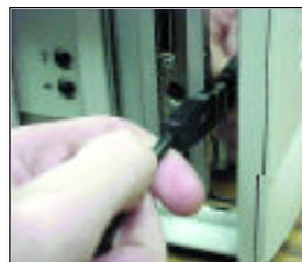
**Note:** The USB connector is designed to fit only one direction. Do not force.
